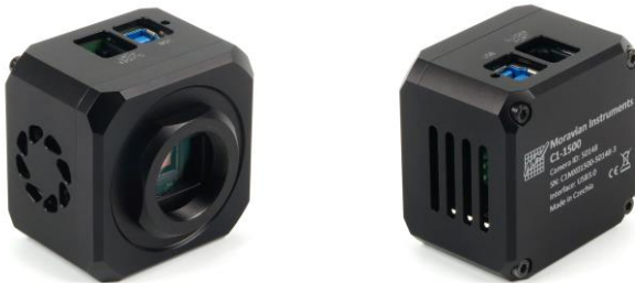
Figure 5: Cooling air intake is on the right side of the C1 camera (left image), while the output vents are on the opposite side (right image)
