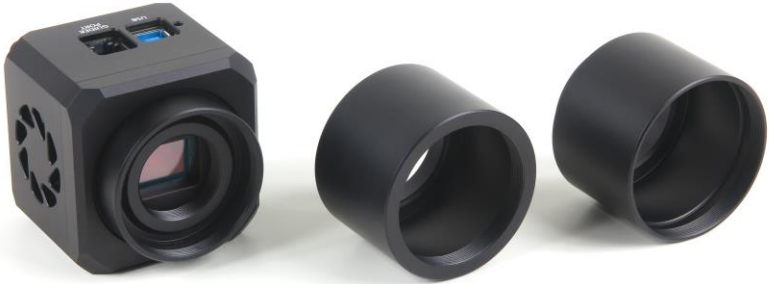
Figure 10: C1 camera (left), 55 mm BFD extension tube with M42×0.75 thread (center) and with M48×0.75 thread (right)
