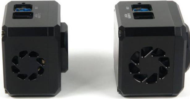
Figure 3: Comparison of the C1 v3 (left) and v1/v2 (right) models shows the difference in camera thickness
